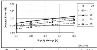
Figure 24. Detector error vs. supply voltage, mode = high
